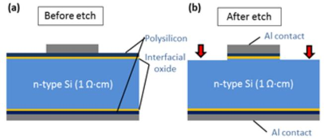
Figure 2: Structure for contact resistivity measurement, (a) before and (b) after modified TMAH etch to stop lateral carrier transport.
