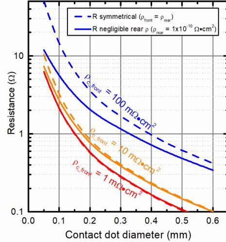
**Figure 4: 3D simulation of C&S dot structure measurements comparing the standard structure of having negligible rear contact resistance to a front-rear symmetrical contact structure.**
