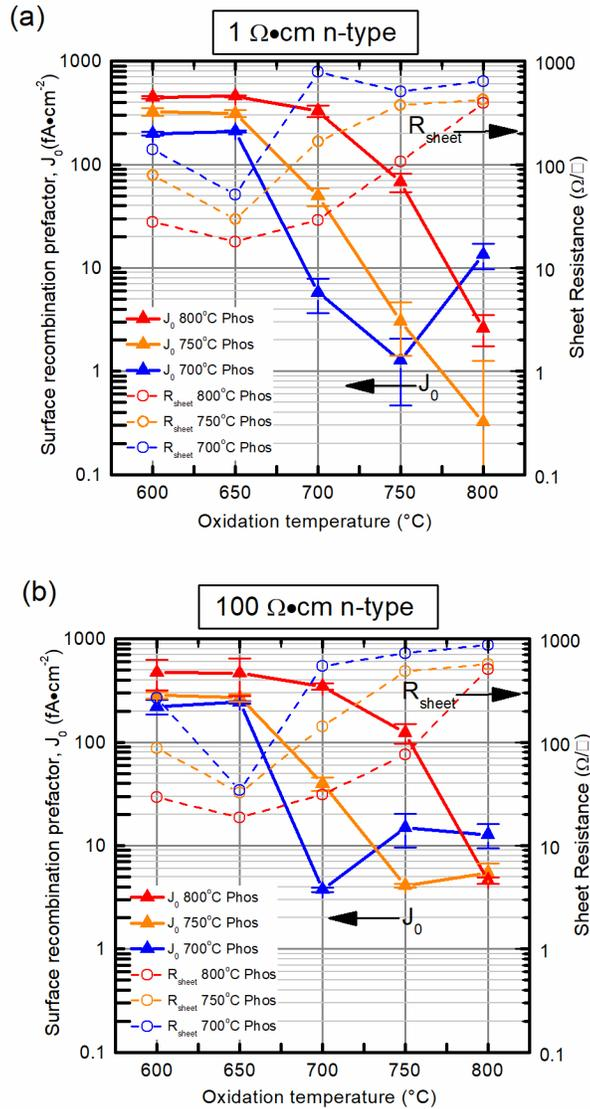
Figure 1:  $J_0$  and  $R_{\text{sheet}}$  versus oxidation temperature for a range of phosphorus diffusion temperature on (a) 1 Ω-cm and (b) 100 Ω-cm n-type wafer.
