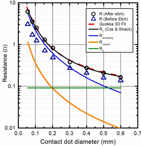
**Figure 3: Comparison of measured resistance before and after TMAH etching to remove polysilicon surrounding contact dots.**
