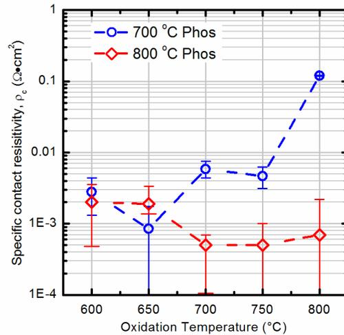
**Figure 5: Deduced  $\rho_c$  from fitting to 3D simulation.**
